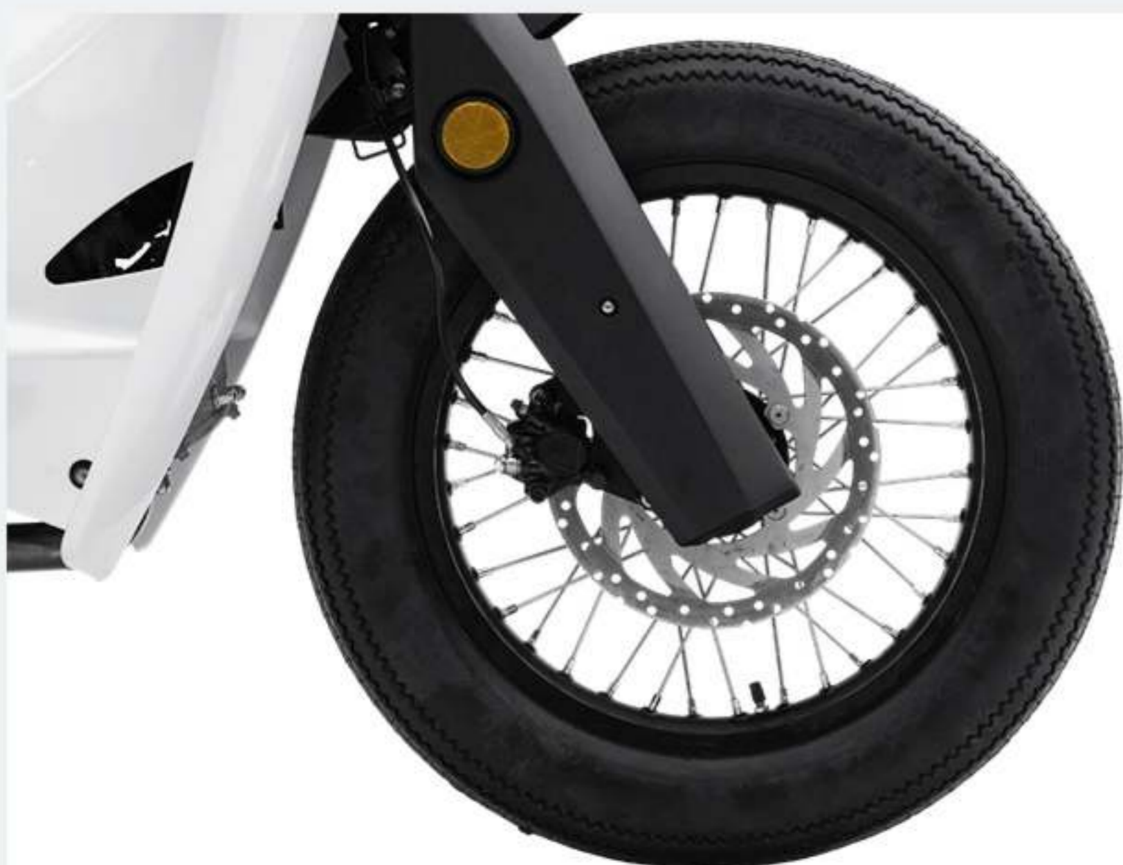
7075 AVIATION ALUMINUM ALLOY WHEEL RIMS WITH STAINLESS STEEL SPOKES
